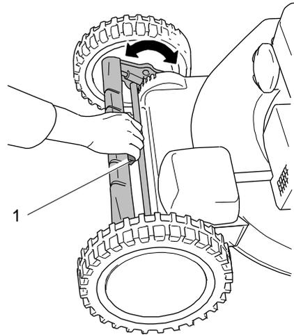
The cutting height can be adjusted on each axle in 6 levels of 30 mm up to 100 mm.
