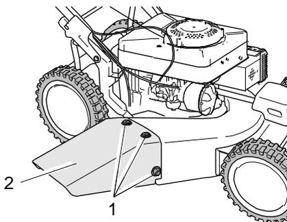
1. Insert the attached 3 cup square bolts with a big washer from the inside of the device housing into the holes (1).
