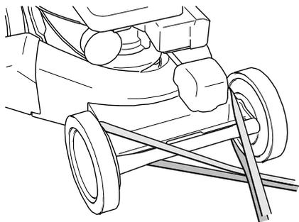
Use tension belts to secure the device.
