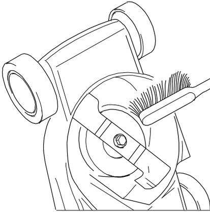
Depending on use, clean the device thoroughly, especially the bottom and the knife.
