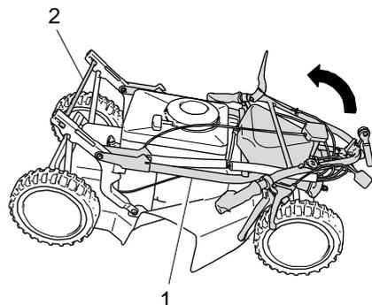
1. Flip the guide bar (1) backwards and engage it with the bar fixing (2).
